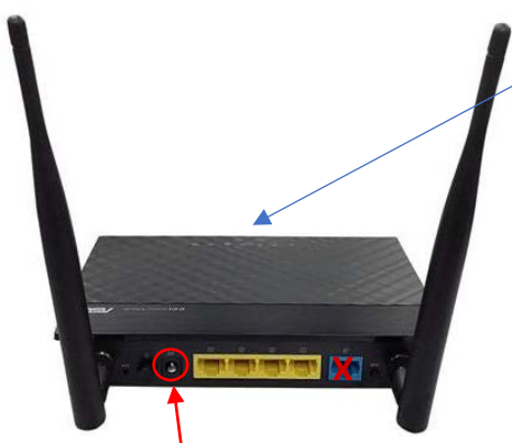
Black Asus Router: The power cord runs from here to the electrical outlet.
